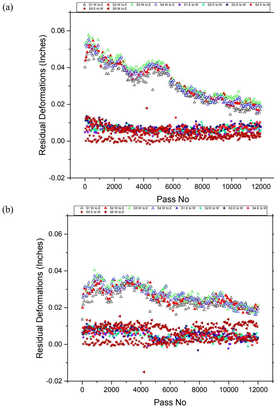
Figure 3: Residual deflections accumulated at wander position 0, a) surface and P209 layers and b) DGA subbase layer
