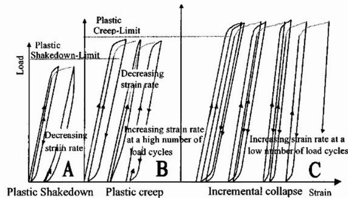
Figure 5: Idealized behavior of granular materials under repeated cyclic pressure load (Werkmeister et al. 2001)
