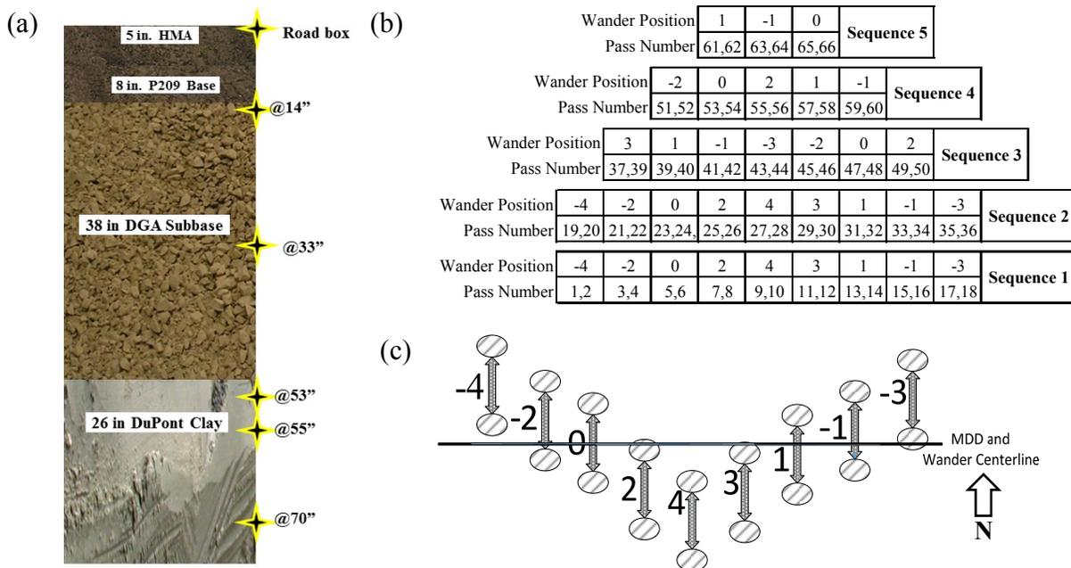
Figure 2. (a) Layer configuration of the dense-graded aggregate (DGA) base, (b) applied wander sequence, and (c) 6-wheel gear centerline position for each wander position
