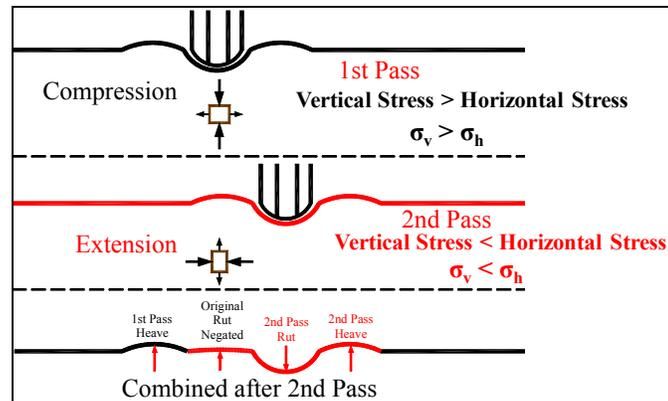
Figure 1. Schematic explaining the rut profile development from an offset wheel
