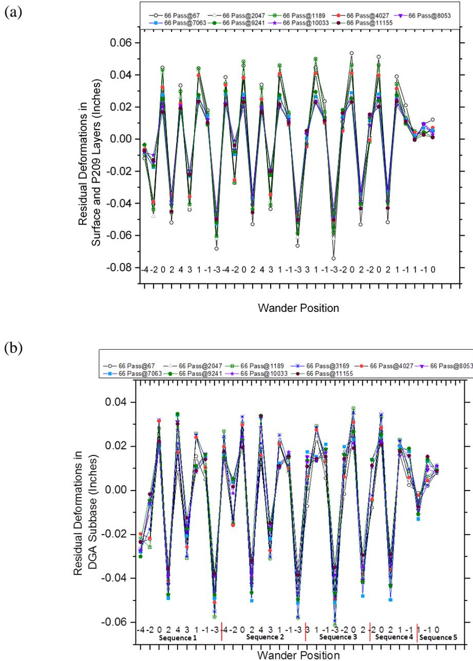
Figure 8: Residual response over 66-pass wander pattern and wander sequence (a) surface and P209 layers (b) DGA subbase layer
