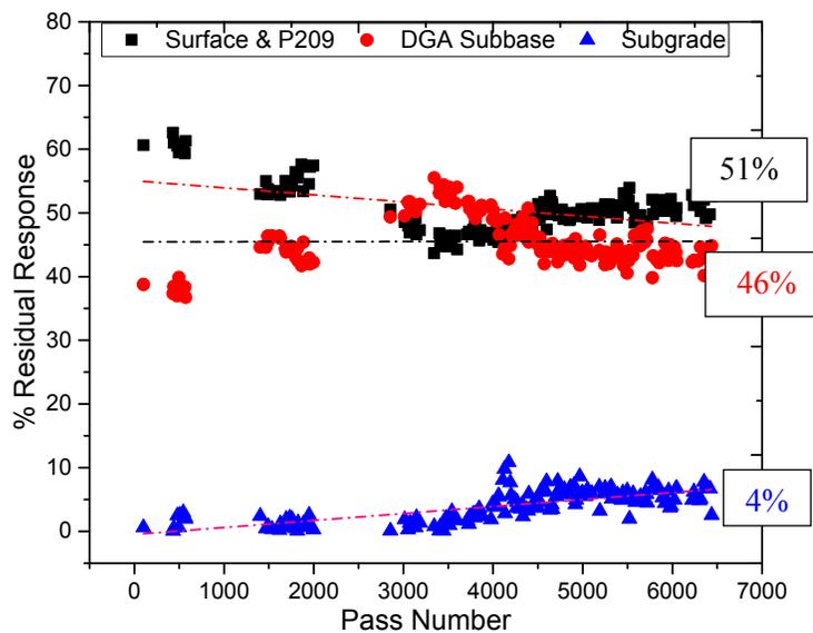
Figure 7: Layer percentage of the total residual response on B777 lane, west to east loading direction, wander position 2
