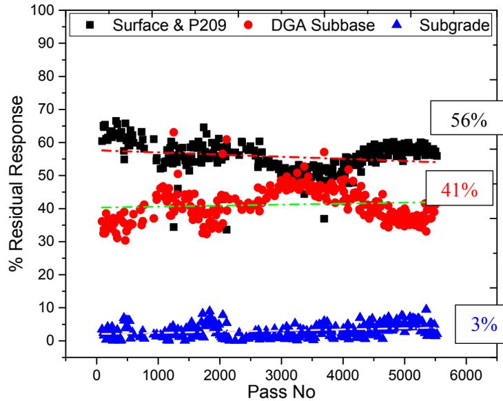
Figure 6: Layer percentage of the total residual response on the B777 lane, west to east loading direction, wander position 0
